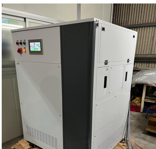
Low temperature vacuum distillation machine Recycling 80-85 %
